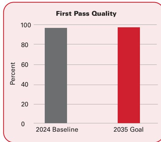
FPQ, also known as throughput yield, is a metric that measures the percent of products manufactured correctly and to specifications the first time through a process, without any rework or scrap.
